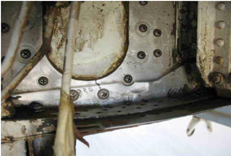
A-4 front spar cracking
