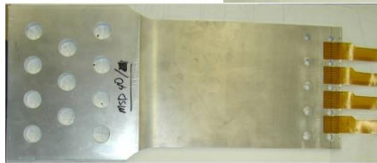
10-Hole Specimen with MWM-Array Networks
