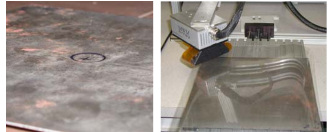
Figure 15. Left: A dented steel plate. Right: Plate with an FA24 MWM-Array and a 0.020-in. plastic sheet.
