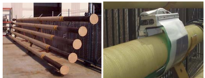
Figure 9. (Left) Simulated PRCI riser samples with embedded corrosion defects. (Right) Photograph of a prototype external scanner on these pipe sections.
