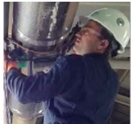
Figure 17. Redeveloped JENTEK MR-MWM-Array sensor, for scanning through-wall and insulation.
