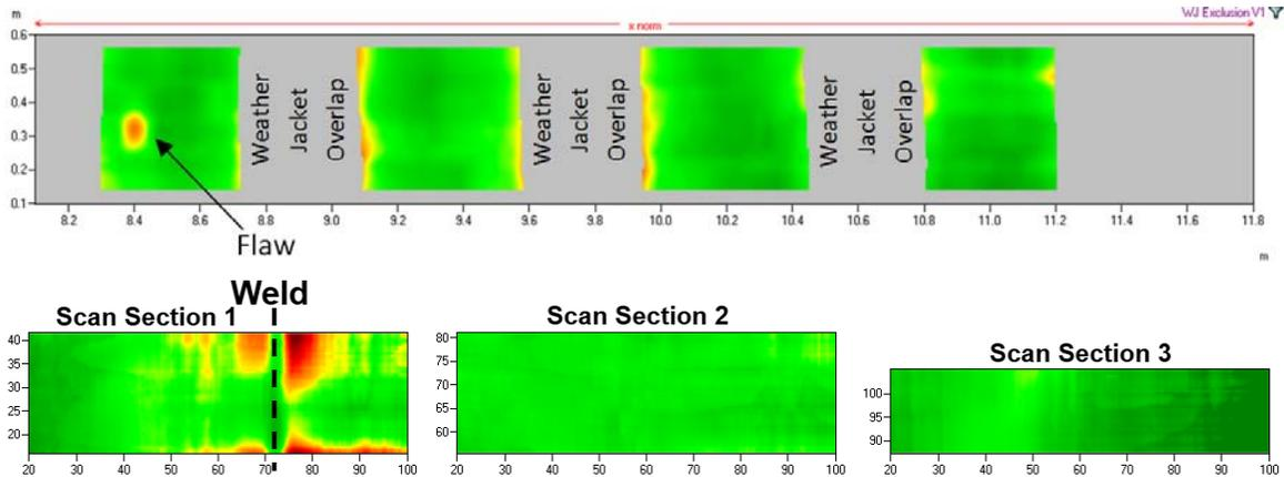
**FIGURE 6.** Pipe wall thickness images are shown above for imaging of corrosion through weather jacket and insulation. (top) Insulation thickness is 2 inches, the weather jacket is 0.5 mm thick aluminum, and the pipe walls are 0.25 inches and the corrosion is external. (Bottom) Insulation thickness is 2 inches, the weather jacket is 0.5 mm thick aluminum, and the pipe walls are 0.5 inches and the corrosion is internal.
