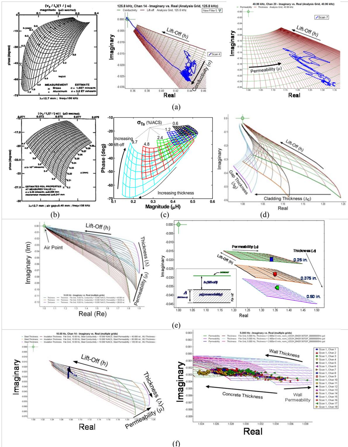
**FIGURE 2.** Grids and Lattices corresponding to schematics from Figure 1, (a) through (f). Grids a(left) and b(left) were generated in 1989 [4,7]. The b(left) grid is for conductivity and thickness. Before this grid is used a higher frequency measurement provides the lift-off in a “hierarchical” 3-unknown inverse method.
