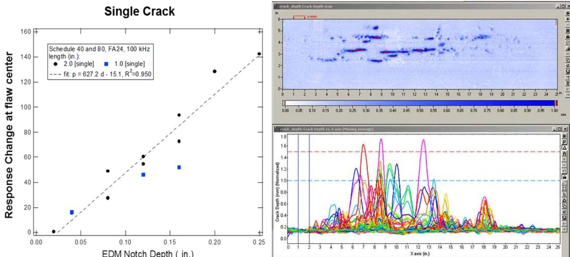
**FIGURE 3.** (left) Data showing magnetic permeability response can also be correlated very well with crack depth; (right) displayed as a C-Scan image of depth for each crack or as a B-Scan for the individual channels.
