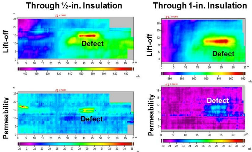
**FIGURE 5.** Images of lift-off (which is the same as the coating thickness in this case) and magnetic permeability for a riser with a relatively insulating coating. Both the lift-off and the magnetic permeability images show the defect, even when the insulating coating thickness is varied without informing the method.
