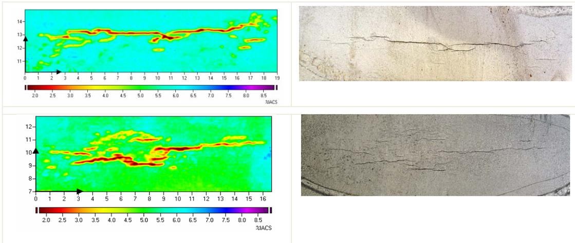
**FIGURE 4:** (left, top and bottom) MWM-Array crack response C-Scan images. (right, top and bottom) corresponding enhanced photographs of the crack morphology.
