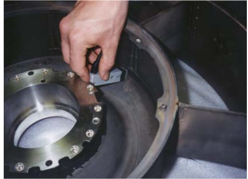
MWM Measurements on the I.D. Surface of the Internal Rim Opposite the Seam Weld
