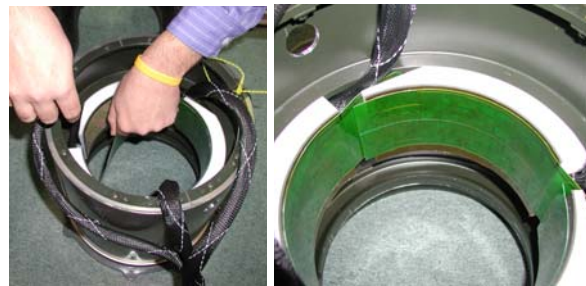
Figure 7. Nine QD-MSGs (3 QD-MSG-Arrays with 3 QD-MSGs each) mounted to a pre-existing assembly installed around an unmodified main rotor shaft in a test cell at Boeing Rotorcraft.
